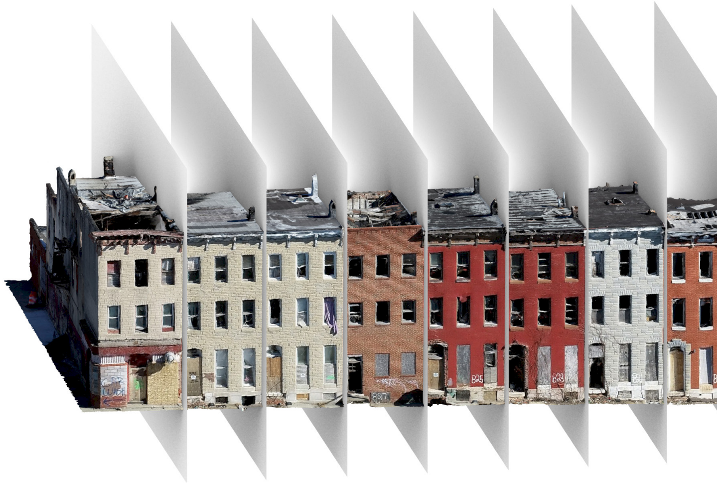
Figure 4. Digital models created from point cloud data, separated into individual units for mass customized retrofit design. Image: Brent Sturlaugson
